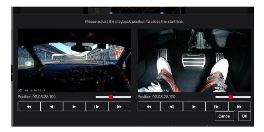
Set the playback position of the displayed image to "position across the starting line". If sub images are loaded, set both images.
